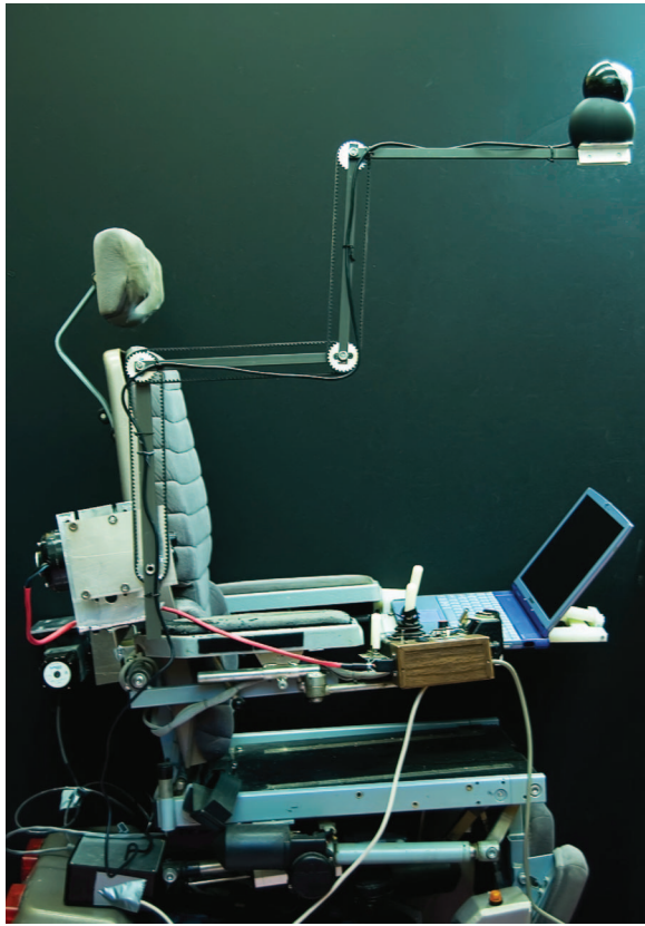
Fig. 3 Lateral view of the prototype WC camera mounted above the armrest of a power wheelchair. This location does not interfere with the movements of a WC user or the functions of the WC. When the device is retracted, the user is able flip up the armrests to transfer from and into the WC. In this view, the device is rotated 90 deg placing the digital camera slightly above eye height.
