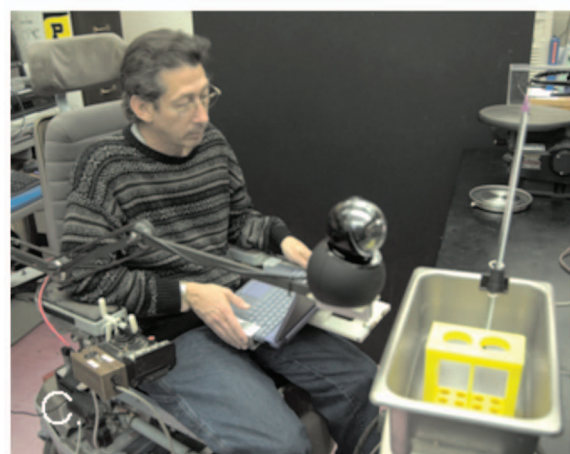
Fig. 2 The body mechanics of sitting in a WC makes forward viewing problematic because of their low height and the difficulty to direct one's eye line at the object of interest. (a) A WC user attempts to peer inside a water bath on a cabinet-style laboratory bench. Without feet and knee clearance, (b) demonstrates the typical sideways posture of a WC user to get close enough to look inside a water bath on a hot plate. This posture can cause neck and back strain over time as well as safety concerns, such as positioning one's face close to the hot water bath. (c) The WC camera permits viewing inside the water bath without having to strain the body to get near. Real-time camera viewing through a laptop PC also permits images and video to be recorded.
