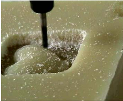
Milling by telescopic drive PKM
