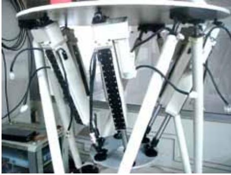
Figure 5. The telescopic drive PKM
