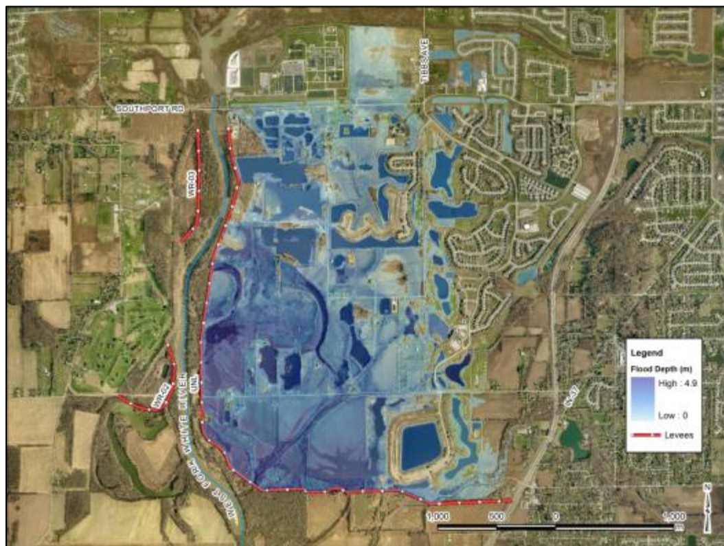
Figure 13: UNL Levee Breach Depth Grid
