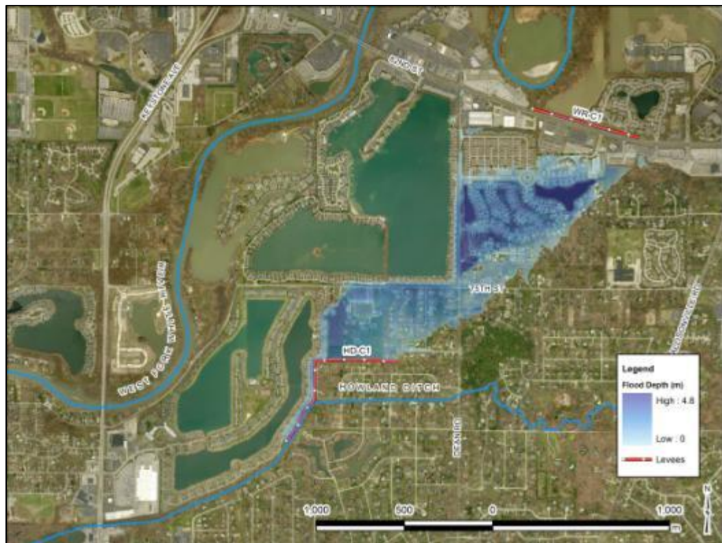
Figure 11: WR-C1 Levee Breach Depth Grid
