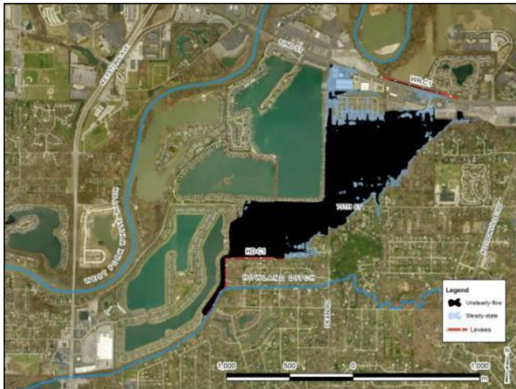
Figure C.2: Unsteady-flow vs. Steady-state Floodplain Boundaries for WR-C1 Levee Breach
