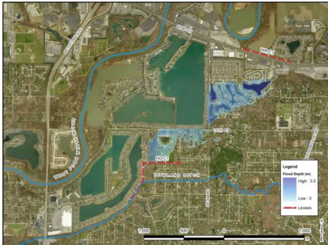
Figure 12: HD-C1 Levee Breach Depth Grid
