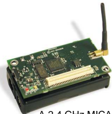
A 2.4 GHz MICAz mote from Crossbow.
