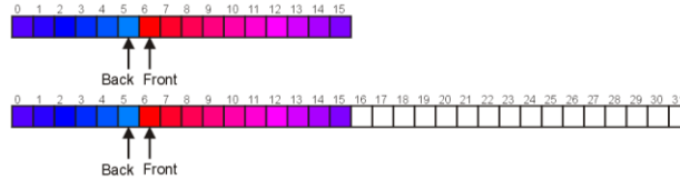
Figure 7. A blind copy of a full array into one with twice the capacity.
