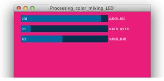
Then add the functionality to send out values from your Processing sketch that control the brightness of each color component in the RGB LED: http://web.ics.purdue.edu/~fwinkler/AD32600\_F14/Processing\_color\_mixing\_LED.zip
