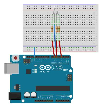
With our RGB LED (Jameco part no. 2125181) use the following resistors: R1, R2 =  $100\Omega$ , R3 =  $150\Omega$  or if you don't have these values R1, R2 =  $100\Omega$ , R3 =  $220\Omega$ .
