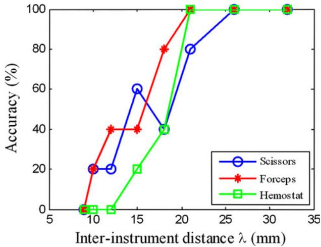
**Fig. 9** Instrument picking accuracy versus inter-instrument distance ( $\lambda$ )
