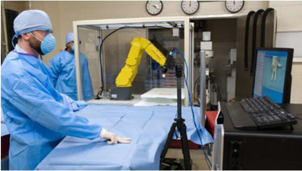
**Fig. 1** The real-time robotic scrub nurse in operation in an OR
