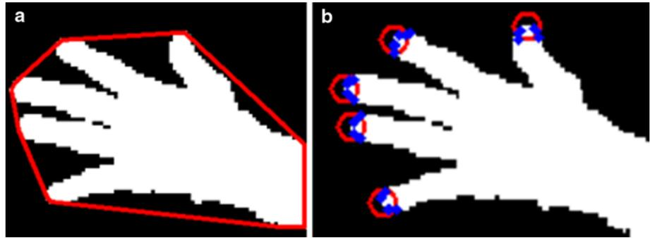
We empirically found that the fingertips lie close to the convex hull  $H$ . Let  $NN(P, H)$  return the nearest neighbor of  $P$  in  $H$ , and let  $d$  be the threshold on the Euclidean distance from the convex hull. We refine the candidate set  $S$  based on the proximity to the convex hull  $H$  and define  $F_C$  as:
