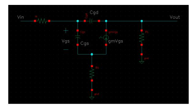
3. The amplifier shown below is biased to operate at Id=1mA and gm=15mA/V. Neglecting ro, find the midband gain. Find the value of Cs that places the corresponding pole at 10Hz. What is the frequency of transfer-function zero introduced by Cs? Give an expression for the gain function.
