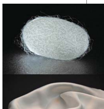
The light strongly scattering from a natural silk cocoon, indicating that silk fibers are natural metamaterials with densely packed nanostructures. Bottom: The brilliantly "white" and "lustrous" reflection of natural silk fabrics without any chemical treatments.
