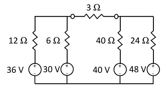
Rewrite each of the resistor/voltage source pairs as parallel resistor/current source pairs with currents of 36/12=3A; 30/6=5A; 40/40=1A; 48/24=2A
