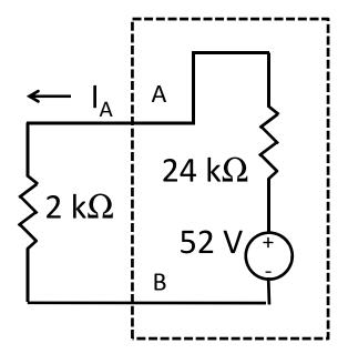
$$R_{th} = \left(\frac{1}{72} + \frac{1}{36}\right)^{-1} = 24 \text{ k}\Omega$$
