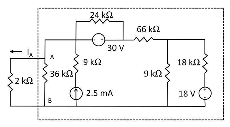
$$R_R = \left(\frac{1}{9} + \frac{1}{18}\right)^{-1} = 6 \text{ k}\Omega; I = 1 \text{ mA; V=6 V}$$
