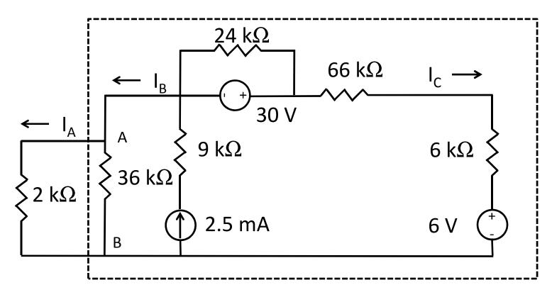
$$R_{th} = \left(\frac{1}{72} + \frac{1}{36}\right)^{-1} = 24 \text{ k}\Omega$$
