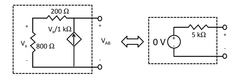
With no independent sources, can be reduced to a single resistor
