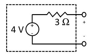
Fitting to  $I_A = \gamma V_{AB} - \sigma$  yields  $\gamma=1/3$ ,  $\sigma=4/3$
