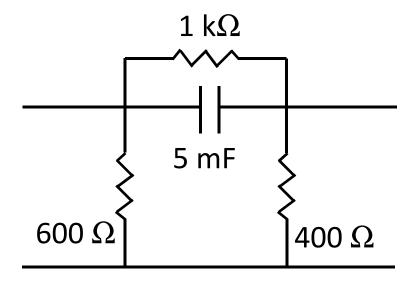
•  $V_C$  for zero input: capacitor sees two resistors of 1 k $\Omega$ ;  $R_{th}$ =500  $\Omega$ :
