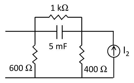
$V_{c}$  from  $I_{2}$  only: source transformation yields  $V_{oc}$ =-10 V; combine series resistors; transform for  $I_{sc}$ =-10 mA;  $R_{th}$ =500  $\Omega$ ; transform again for  $V_{oc}$ =-5 V. With  $\tau$ =(5 mF)(500  $\Omega$ )=2.5 s, we obtain:
