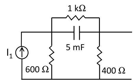
$V_{\rm C}$  from  $I_{\rm 1}$  only: source transformation yields  $V_{\rm oc}$ =30 V; combine series resistors; transform for  $I_{\rm sc}$ =30 mA;  $R_{\rm th}$ =500  $\Omega$ ; transform again for  $V_{\rm oc}$ =15 V. With  $\tau$ =(5 mF)(500  $\Omega$ )=2.5 s, we obtain:
