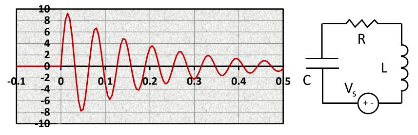
• Combining our previous results of  $L \approx 0.109$  and  $\omega' \approx 100$ , and noting  $Q \gg 1$ , we can estimate  $\omega' \approx \omega_o$ . Since  $\omega_o = \frac{1}{\sqrt{LC}}$ ,  $C = 1/(L\omega_o^2) \approx 1/(0.109 \cdot 100^2) \approx 0.92 \text{ mF}$
