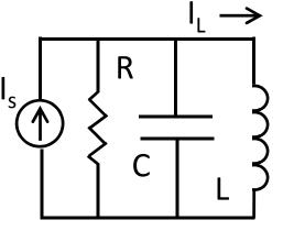
$\Gamma = 1/(2RC); \ \omega_o = 1/\sqrt{LC}; \ \omega' = \sqrt{\omega_o^2 - \Gamma^2} = -i\Gamma'$
