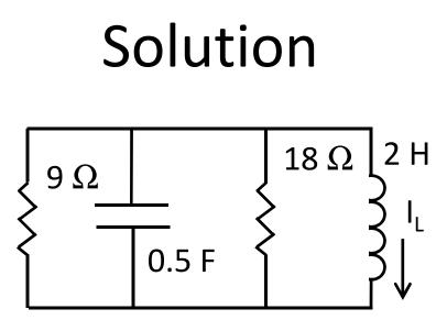
• Ignoring voltage source, circuit reduces to parallel RLC circuit, so that  $\Gamma = \frac{1}{2RC} = \frac{1}{2 \cdot 6\Omega \cdot 0.5 F} = 1/6$ ;  $\omega_o = \frac{1}{\sqrt{LC}} = \frac{1}{\sqrt{2 H \cdot 0.5 F}} = 1 \text{ rad/s}$ ;  $\omega' = \sqrt{\omega_o^2 - \Gamma^2} = \sqrt{1 - (1/6)^2} = \sqrt{35}/6 \text{ rad/s}$
