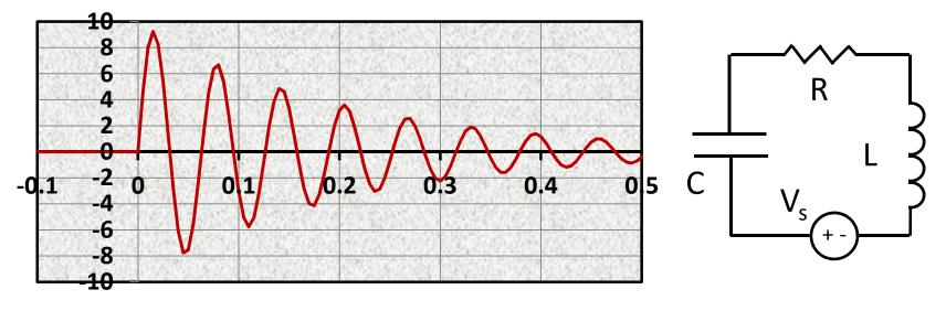
• Recall that underdamped RLC circuits obey:  $V_C(t) = e^{-\Gamma t} \cos(\omega' t + \phi) + V_s$
