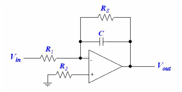
Revised integrating circuit provides shunt resistor to prevent charge storage, plus R<sub>2</sub> to prevent input DC bias current
