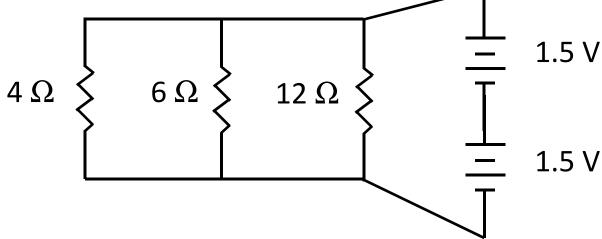
$$I = V_{eff}/R_{eff} = (1.5 + 1.5 V)/2 \Omega = 1.5 A$$
