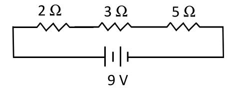
$$I=V/R_{eff}=(9 \text{ V}) / (10 \Omega) = 0.9 \text{ A}$$
