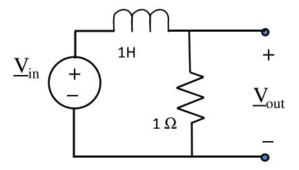
Step 1: Find the impedance of inductor and resistor pair.
