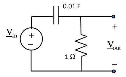
Step 2: Use voltage division to establish output to input ratio.
