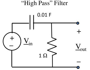
Two plots, one for magnitude and one for phase angle, are needed because  $H(j\omega)$  is a complex quantity.
