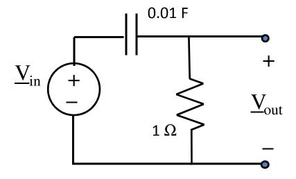
Step 1: Find impedance of the capacitor and resistor pair.
