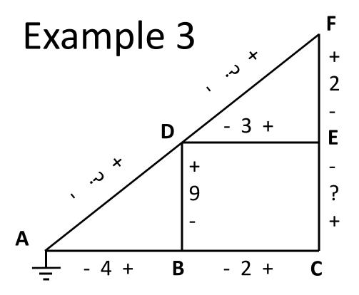
• What are  $V_{DA}$ ,  $V_{FD}$ , and  $V_{EC}$ ?
