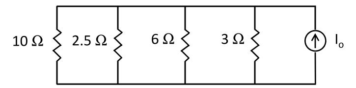
What if 2 identical ICS's are connected in parallel? In series? What if only one has its current doubled?
