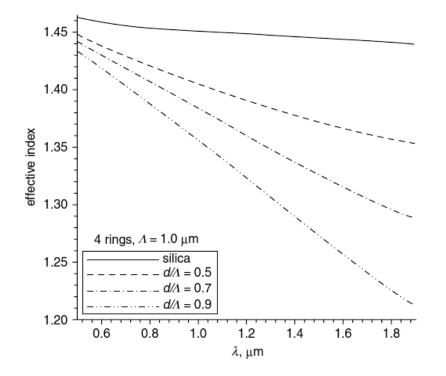
• Calculated dispersion relation (effective index versus wavelength) for a PhC Fiber
