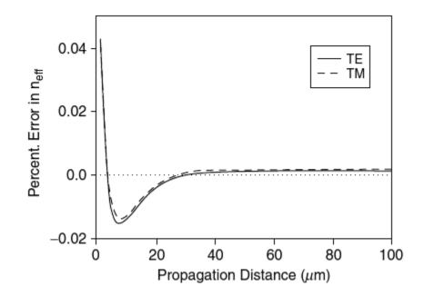
With optimal step size, can solve the fundamental mode of both polarizations in a pretty modest number of steps!
