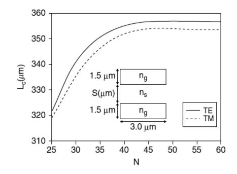
• Accuracy of calculation of waveguide coupling length as a function of mesh divisions *N*
