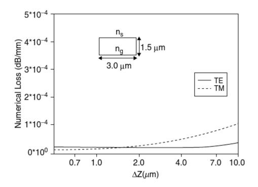
• Propagation step size in Z, known as  $\Delta Z$ , should equal transverse dimensions for best accuracy
