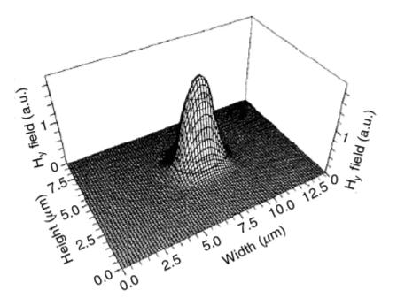
• Fundamental mode is calculated accurately with 12,800 first-order triangular elements
