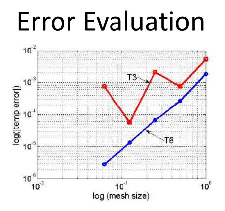
Error for linear elements T3 higher overall than quadratic elements T6; both decrease almost quadratically with mesh size
