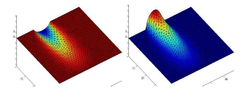
Steady-state solution for a thermally insulating medium, with a variable temperature placed along one surface
