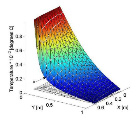
Steady-state thermal gradient between two adjoining walls with different temperatures
