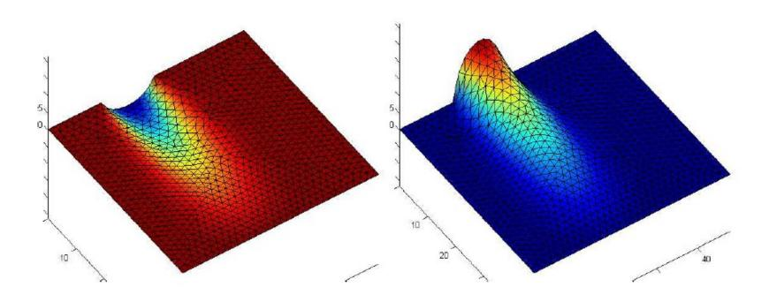
Steady-state solution for a thermally insulating medium, with a variable temperature placed along one surface
