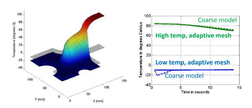
Transient cooling of a shrink-fitted assembly
