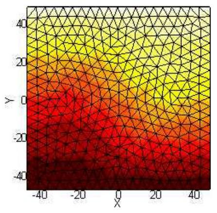
Steady-state solution for heat diffusion in an inhomogeneous medium
