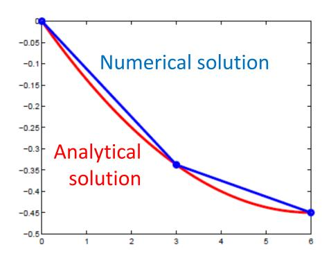
Numerical solution matches analytical solution closely at key
