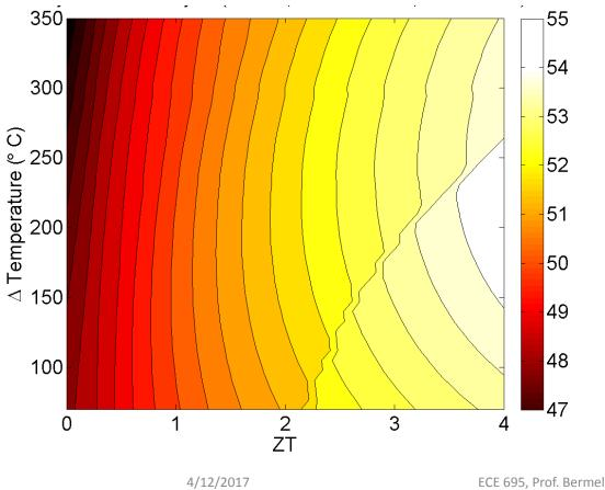
Calculated system exergy as a function of the selective solar surface (SSS) temperature differential (75-350  $^{\circ}$  C) and the ZT value of the thermoelectrics. We assumed 500x solar concentration. As one goes from no thermoelectrics to ZT=4, an overall improvement of 8% can be achieved. These calculations take into account reradiation losses at high SSS temperatures
