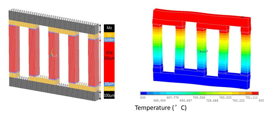
Thermomechanical 2D simulation for a 5-leg TE module in ANSYS. The TE material is SiGe, and the substrates are Molybdenum. The largest stress at interfaces is on the order of 56 MPa ( $\Delta$ T = 170 °C) in share stress (horizontal-direction)
