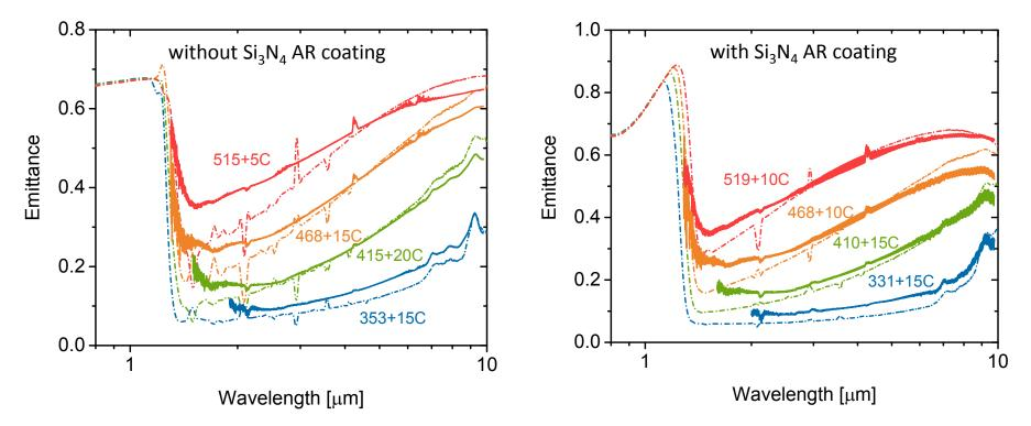
High spectral selectivity is observed at 468 °C in both samples, with a cutoff wavelength of approximately 1.3  $\mu$ m. Higher short-wavelength emittance is both predicted and observed for the structure with a Si<sub>3</sub>N<sub>4</sub> AR coating
