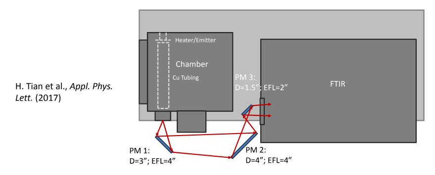
The sample is heated by the heater, and the emitted light is collected and guided by the Cu tube, transmitted through a CaF<sub>2</sub> window, reflected by three off-axis parabolic mirrors (PM 1, 2, and 3, Edmund Optics) to a Fourier Transform InfraRed (FTIR) spectrometer with a mercury cadmium telluride detector and KBr beam splitter (Thermo Fisher Nicolet 670).
