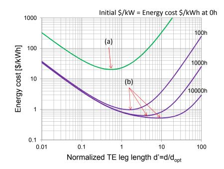
Energy cost vs. normalized leg length, assuming the same parameters as before. Thicker TE legs cause higher efficiency but reduced power output. The economical optimum exists in between the design for maximum power output and maximum efficiency.
