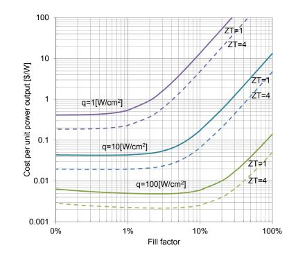
Cost per power output \$/W as a function of fill factor for ZT=1 and 4, and heat fluxes which reflect the heat sink performances. This graph assumes a maximum temperature of 2300K and ambient temperature of 310K, with the TE material price \$500/kg, and substrate \$26/kg.
