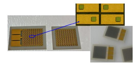
400 elements of 200 n-ErAs:InGaAlAs and 200 p-ErAs:InGaAs elements, 10  $\mu$ m thick, were bonded on the upper and lower AlN plates via wafer scale approach and flip-chip bonding technique.
