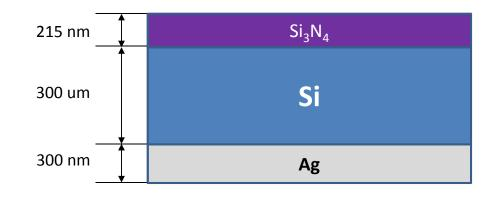
Schematic of the structure for selective absorber based on Si substrate with 215nm  $Si_3N_4$  front antireflection coating (ARC) and 300nm Ag back reflection layer. Heights are not to scale.
