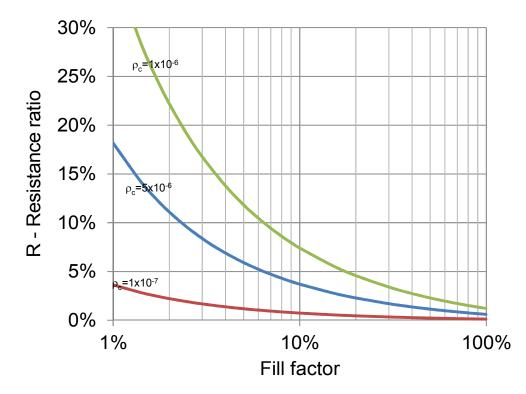
Ratio of parasitic electrical resistance to entire resistance as a function of Fill factor, with a variation of specific contact resistivity [Ohm.cm<sup>2</sup>]. Conditions are for 1000 elements per 1cm<sup>2</sup> module.
