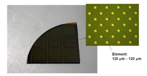
Six full element array chips were fabricated on the quarter wafer. Each element array chip contains 200 elements, and area size of each element is 120  $\mu$ m × 120  $\mu$ m.
