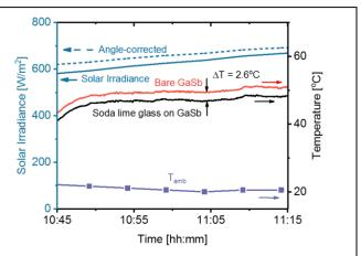
Fig. 3: Daytime radiative cooling measurement on June 7, 2017. Solar irradiance, measured by a pyranometer mounted at 45° facing south (blue solid line) is angle-corrected to quantify the solar irradiance upon a horizontal surface (blue dashed line). Ambient temperature (purple line) is measured by a thermometer sitting below the setup. The stabilized temperature difference between GaSb PV diodes with and without soda lime glass is 2.6 °C.
