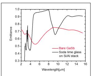
Fig. 2: The mid-IR emittance spectra of bare GaSb (red line) and the soda lime glass (black line). Both are measured by FTIR at a 30° incident angle. The spectrum of soda lime glass is measured when stacked on a Si wafer with aluminum deposited on the back. In the mid-IR, soda lime glass is mostly opaque.
