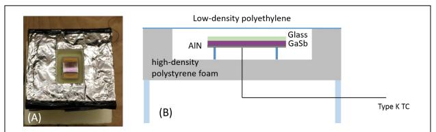
Fig. 1: (A) Radiative cooling test chamber, with 550 μm soda lime glass atop a GaSb PV cell inside.
