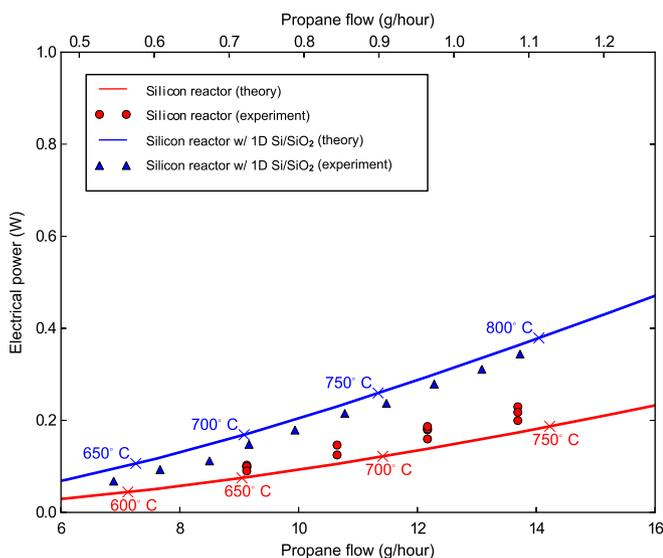
**Fig. 3.** Theoretical and experimental performance of our TPV system with two emitters: bare Si and 1D Si/SiO<sub>2</sub> photonic crystal. Calculated microreactor temperatures are labeled.
