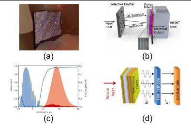
Fig. 1: Potential applications for selective enhancement of thermal emission include: (a) photovoltaics [3], (b) thermophotovoltaics (TPV) [6], (c) selective solar absorbers [4], and (d) photon-enhanced thermal emitters (PETE) [7].
