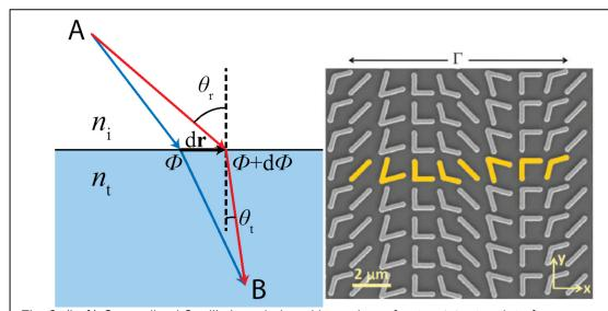
Fig. 2: (Left) Generalized Snell's Law, induced by a phase front  $\Phi(r)$  at an interface. (Right) Metasurface fabricated by Nanfang Yu *et al.*, demonstrating Generalized Snell's law behavior at infrared wavelengths (adapted from [13]).
