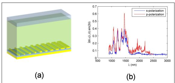
Fig. 4: (a) Xylophone meta-mirror structure for selective enhancement of thermal emission for a partially selective dielectric above with an anti-reflection coating on top. (b) Angle-averaged emissivity for s- and p-polarizations. The s-polarization shows particularly high selectivity for selective thermal emitter applications.
