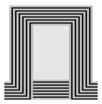
Fig.1 The illustration of the Photonic Crystal (PC) cladded waveguide, with low index core  $(SiO_2)$  and  $Si/Si_3N_4$  as dielectric cladding layers.
