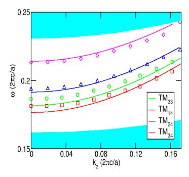
Fig.2 Dispersion relation for modes within the band gap of an on-chip PC cladded waveguide with a core of size 8a by 8a (a is the unit length of the cladding),  $n_{core} = 1.46$ , numerical data (dotted lines) from time domain calculations at specific  $k_{\epsilon}$  values are compared to the metallic waveguide (solid lines). TE modes are nearly degenerate with TM modes.
