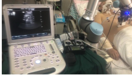
Fig. 3. The Medical Care Module during a trial in Beijing Ditan hospital. The robot was performing ultrasound diagnosis through augmented teleoperation. The monitor is set up for the assistant nurse, who applies the ultrasound gel, and takes over the robot with a radio control in case of emergency.
