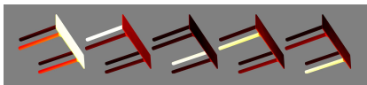
Fig. 4: NMF basis functions ( k = 5 ) for the table mesh. The table top and each leg are isolated in different functions.
