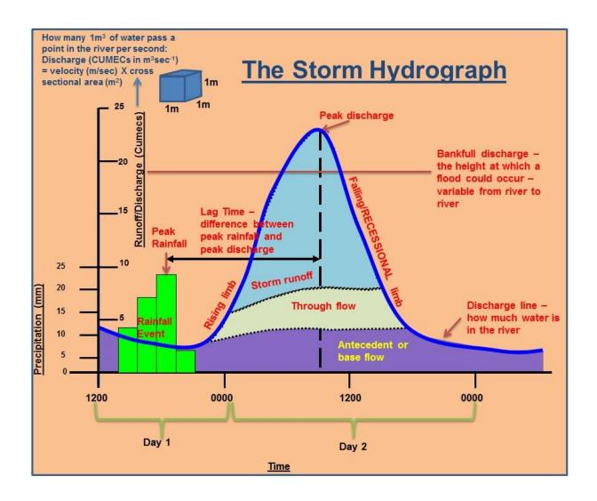
Rainfall hyetograph creates a discharge hydrograph at the receiving stream or watershed outlet
