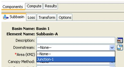
You will see that a link (line) will appear in the basin model to show the connectivity between subbasin-A and Junction-1. Similarly, link Subbasin-B with Junction-1. Save your project. Your final HMS-schematic should show both sub-basins connect at the junction as shown below.
