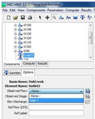
Run the model again, and see the results at Outlet3. You will now see both the model hydrograph and observed hydrograph.
