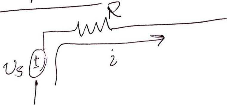
$$\begin{aligned} \text{instantaneous power: } p(t) &= i(t)v(t) \\ &= \frac{1}{R}v^2(t) \end{aligned}$$
