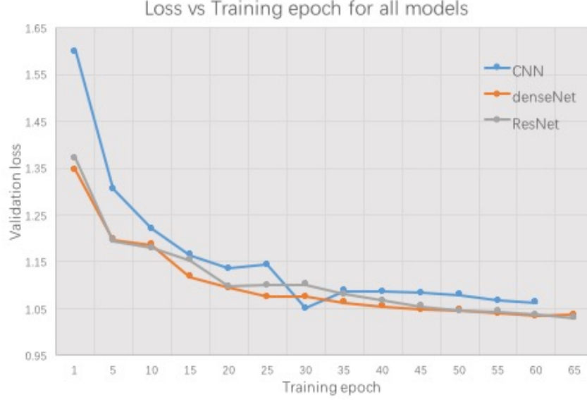
Fig. 3.16. Validation loss descents quickly in all three models, but losses of DenseNet and ResNet reach plateau earlier than that of CNN
