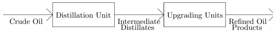
Figure 1: Refinery Process Flow Chart. Source: Simplified illustration based on Gary et al (2007).
