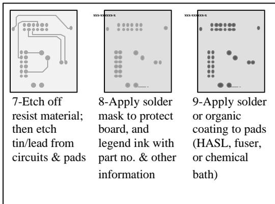
Figure 2-3. The finishing steps PCB fabrication.
