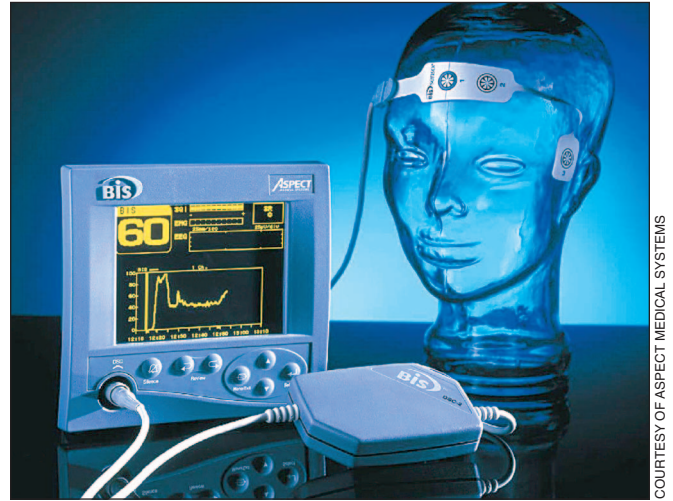
Figure 2. Bispectral index (BIS) monitor. A sensor is placed on the patient's forehead to measure electrical activity in the brain and monitor the patient's level of consciousness.
