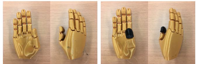
Figure 1: 3D printed Flex-Hand model for the handshake (Left) and object grasp (Right) experiment. A thumb angle of the hand is different because the position of the thumb changes depends on the various task.
