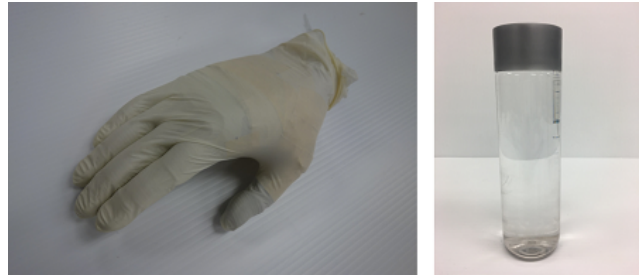
Figure 2: A fixed Flex-Hand for handshaking (Left) and a cylindrical water bottle for object grasping (Right). For the purpose of maintaining even coverage of black ink to remain on the surface across multiple trials, a disposable latex glove was used on the Flex-Hand.
