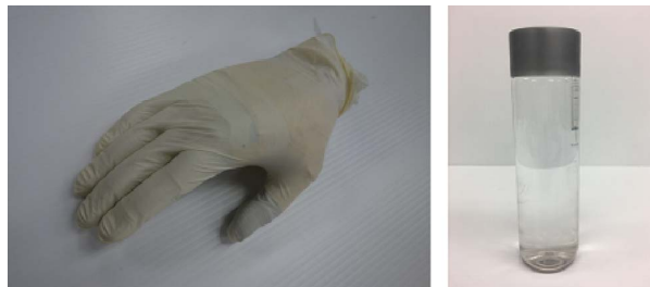
Figure 2: A fixed Flex-Hand for handshaking (Left) and a cylindrical water bottle for object grasping (Right). For the purpose of maintaining even coverage of black ink to remain on the surface across multiple trials, a disposable latex glove was used on the Flex-Hand.
