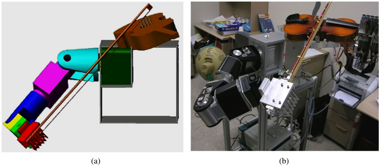
Fig. 4 a A model of the violinist robot simulated in SolidWorks. b The external appearance of the developed violin playing robot named “Violinist Robot”
