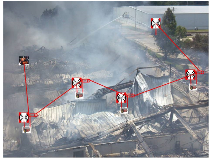
Fig. 14. Firefighting robot linked to base station through a set of follower robots
