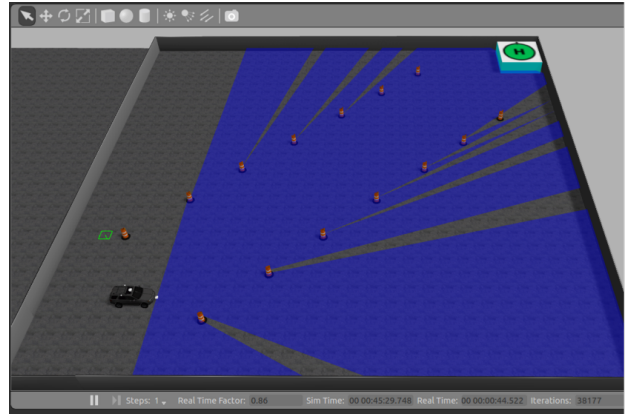
(b) Gazebo simulation environment. A vehicle follows the desired path which is a straight line from the initial location at the bottom left to the home at the top right.
