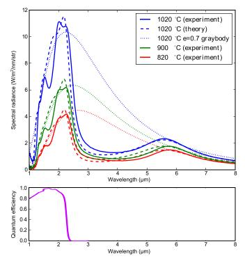
**Fig. 4.** (*Upper*) Measured and simulated thermal emission, normal to the surface, of the photonic crystal at 820, 900, and 1,020 °C plotted with solid and dashed lines, respectively. Simulation results of three graybody emitters with 0.7 emittance (approximation of Si emittance), at 820, 900, and 1,020 °C are shown with dotted lines. (*Lower*) Measured external quantum efficiency (EQE) for the GalnAsSb PV cell with antireflective coating.
