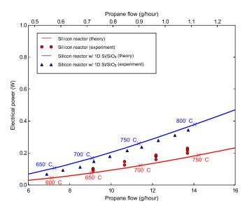
Fig. 3. Theoretical and experimental performance of our TPV system with two emitters: bare Si and 1D  $\text{Si/SiO}_2$  photonic crystal. Calculated microreactor temperatures are labeled.
