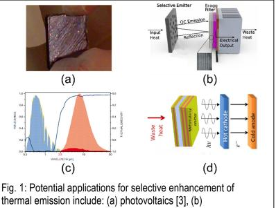
thermophotovoltaics (TPV) [6], (c) selective solar absorbers [4], and (d) photon-enhanced thermal emitters (PETE) [7].
