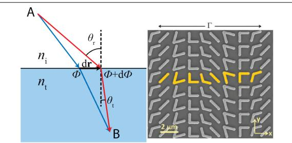
Fig. 2: (Left) Generalized Snell's Law, induced by a phase front  $\Phi(\mathbf{r})$  at an interface. (Right) Metasurface fabricated by Nanfang Yu *et al.*, demonstrating Generalized Snell's law behavior at infrared wavelengths (adapted from [13]).
