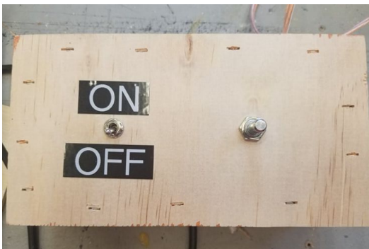
Figure 13: Box to control speed and turn machine on
