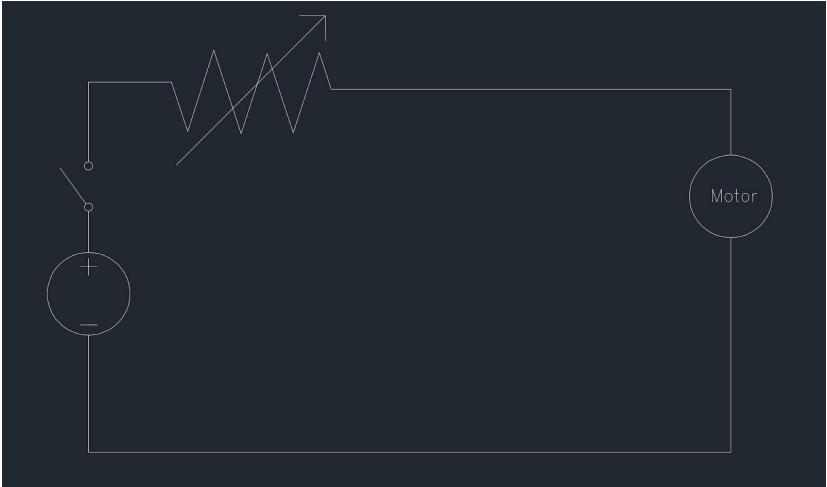
Figure 8: Wiring diagram for drop device
