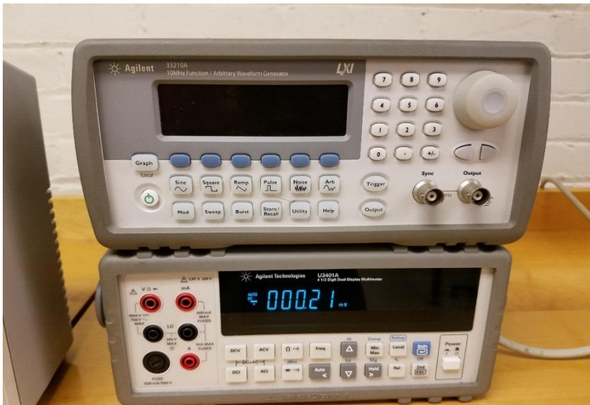
Figure 1: The DMM (bottom) is in the middle of your lab station, underneath the waveform generator (top).
