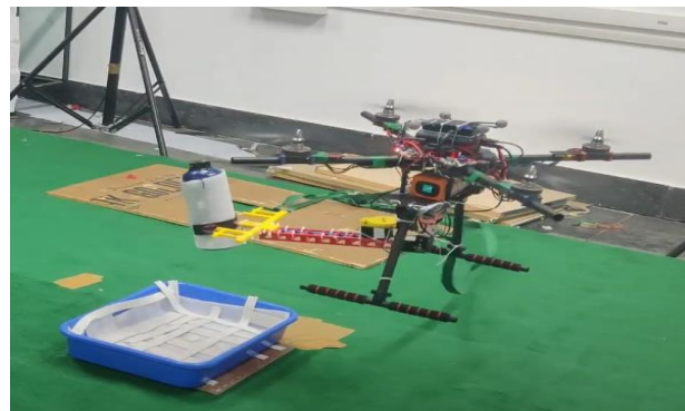
Fig. 2: Developed Prototype performing grasping and object manipulation operation.
