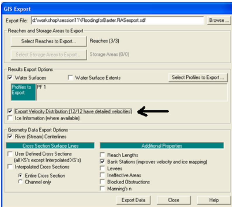
After the data are exported to a .sdf extension GIS file, follow the instructions on Page 29-32 to import the sdf file data into ArcGIS to create a flood inundation map.
