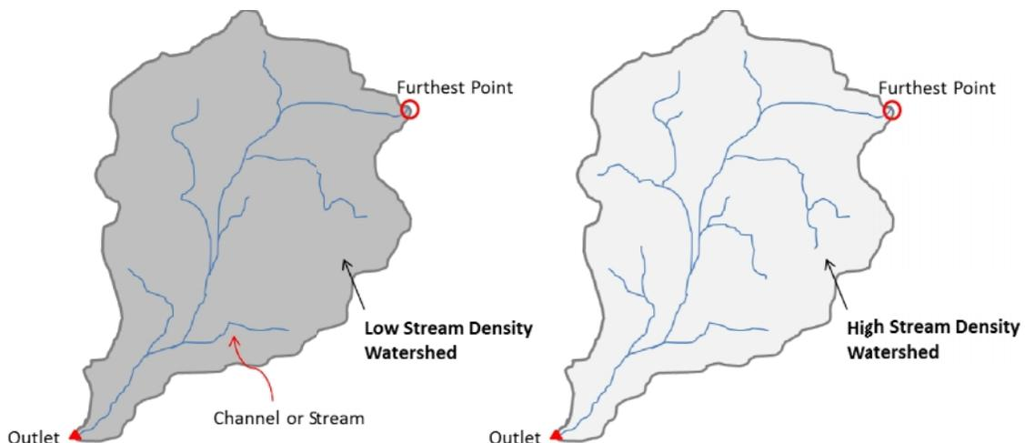
A watershed with large number of tributaries has higher drainage density than a basin with very few tributary streams. The figure above shows example of two watersheds having different drainage density, assuming all other properties (area, surface imperviousness, slope etc.) to be the same.
