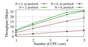
Figure 7: Effect of prefetching on throughput
