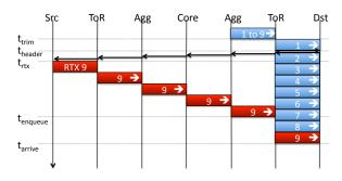
Figure 3: Packet trimming enables low-delay retransmission
