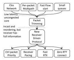
Figure 1: Key components of NDP
